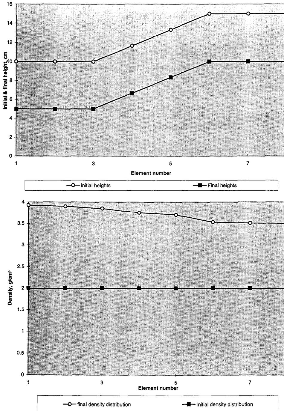
Fig. 7. Calculation results for pressing the article with a stepped-inclined surface.
