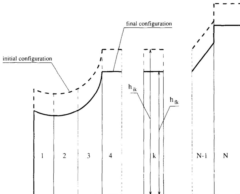
Fig. 1. Subdivision of a characteristic cross-section into elements.
