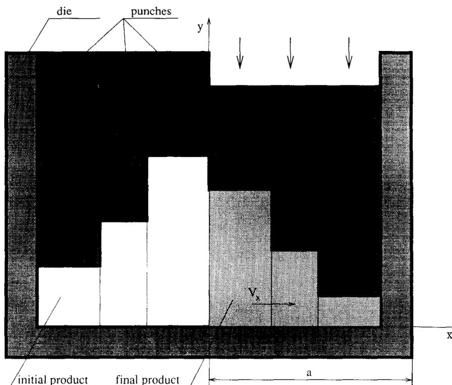
Fig. 3. Schematic of pressing of a stepped article.
