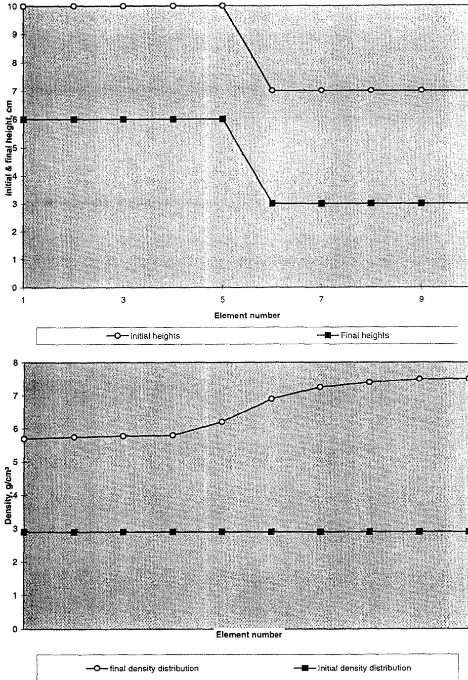
Fig. 6. Calculation results for pressing the stepped article by a single punch.
